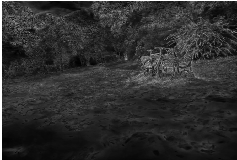
Figure 5.6: Debug render displaying the number of splats contributing to each pixel. Fully white means 255 or more splats contribute to that pixel. Fully black mean there are no splats contributing to that pixel. The maximum contribution was 271.
